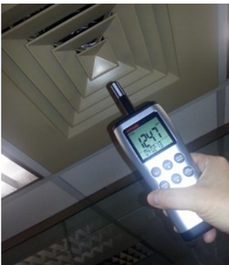
CP11: For mobile fast and reliable measurement of the relevant IAQ
