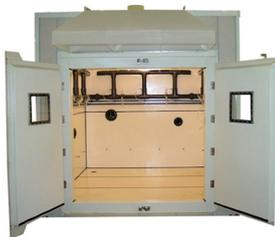
The Saltwater-Spray-Test is the most used method of an accelerated corrosion measuring operation.
