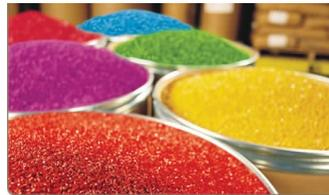
as reduced tensile and impact strengths. Polyamide for example is one of the most hygroscopic plastic materials in common use. The moisture content of nylon molding resins is a particularly important parameter with a direct effect on molding, mechanical properties, viscosity of the melt and the appearance of the molded parts. All plastic producers have to realize the importance of proper drying for molding high quality products!
