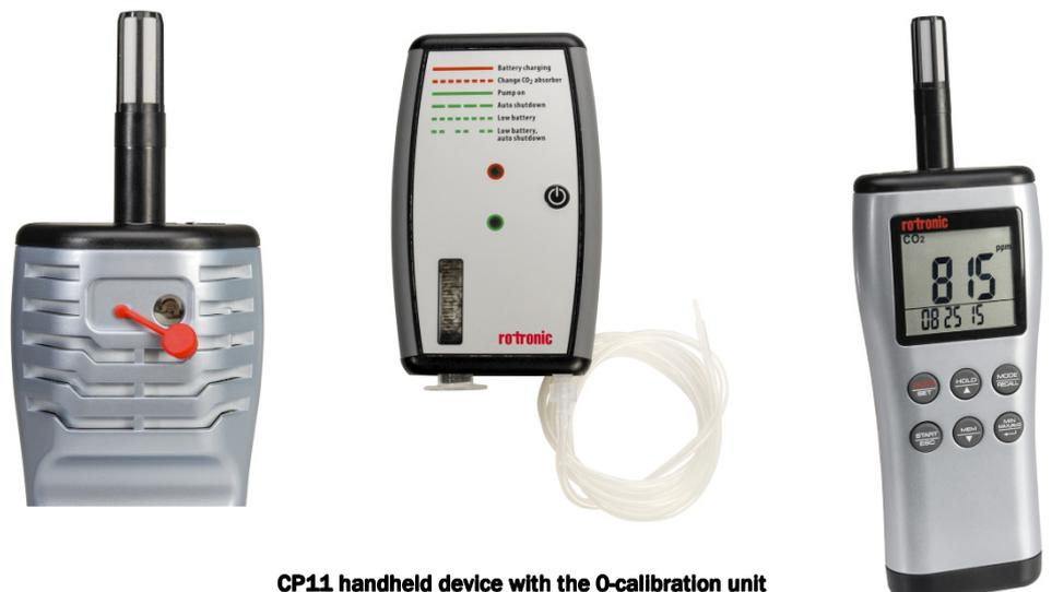
CP11 handheld device with the 0-calibration unit
